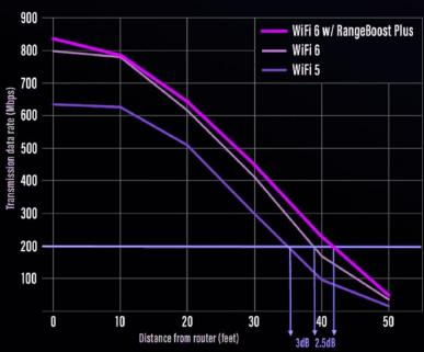
Tests performed in an obstruction-free environment using 80MHz channels.
